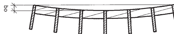
Concave deviation oq max. = 1/200 th of width for dimensions > 600 mm; max. 8 mm smaller dimensions than 600 mm; max. 3 mm
